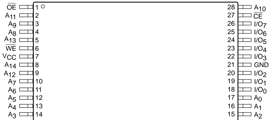
TSOP Top View (8mm X 13.4mm) (H13)
